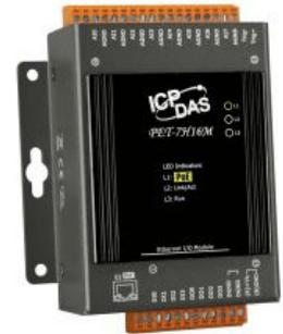
The module provides a programmable input range on all analog Input channels, and the Digital Output can be set to output with short-circuit and overload protection. The PET-7H16M series also provides 4 kV ESD protection as well as 2500 VDC intra-module isolation.
