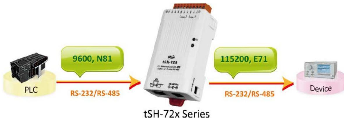
If the device(s) are centralized, you can use a 2<sup>nd</sup> TSH-725 afterwards to change the baud rate back or you can use an I-7514 which is an active star hub which allows for different baud rate setting for each RS-485 output channel.
