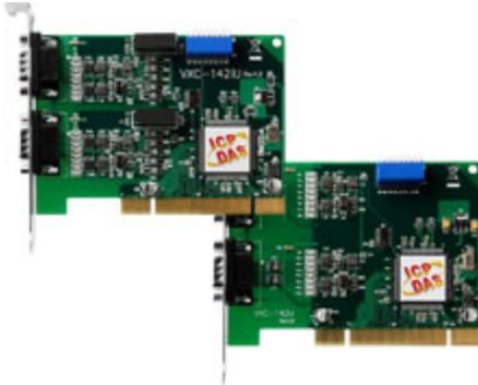
The VXC-142 plugs directly into a PCI slot on any Windows or Linux PC listed in the supported drivers. For Windows, this provides a plug and play solution. Each card contains 2 RS-485 ports with DB-9 connectors. These boards also work with both 3.3 and 5.0 VDC PCI bus types
