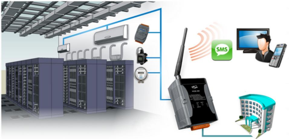
Finally, WISE-5801 allows for external control and monitoring by SCADA software. This enables the collection of power consumption and other data for statistical analysis which leads to improved costs and efficiency over time.
