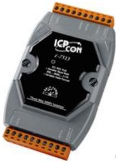
Our I-7513 is a 3 way repeater which allows for branching of the RS-485 signal in 2 or 3 directions. This is ideal for situations where either the signal strength has become too weak or where the slave devices are not placed where a single bus is practical.
