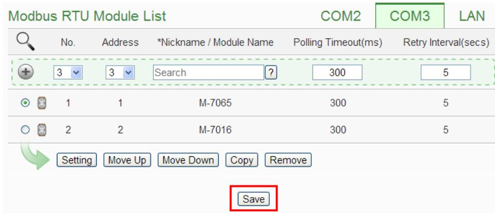
**Please note:** if fail to scan the I/O modules, please make sure the RS-485 cable is properly connected. And then go to [Step 1](#): “System Setting”→”I/O Interface Setting” to make sure the settings of the COM Port that are connected to the I/O Module are accurate. After all settings are completed, click “Save” button to save the changes and repeat [Step 3.1](#) to perform scanning of the I/O modules again.
