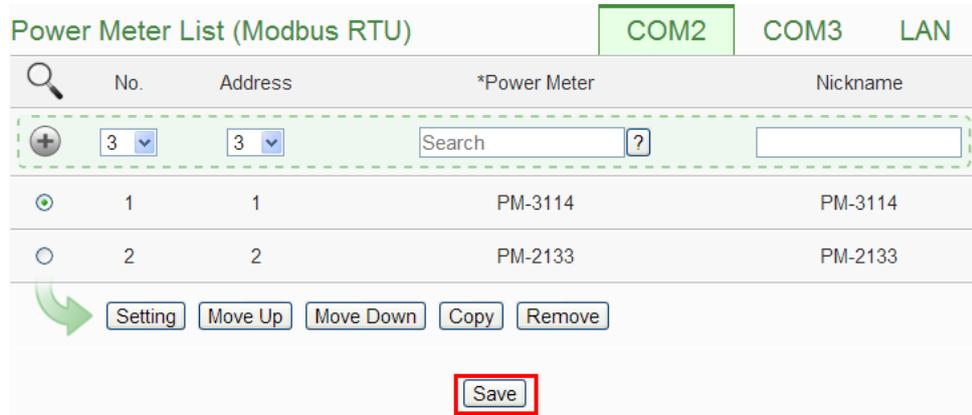
**Please note:** if fail to scan the power meters, please make sure the RS-485 cable is properly connected. And then go to [Step 1](#): “System Setting”→”I/O Interface Setting” to make sure the settings of the COM Port that are connected to the power meter are accurate. After all settings are completed, click “Save” button to save the changes and repeat [Step 3.1](#) to perform scanning of the power meters again.
