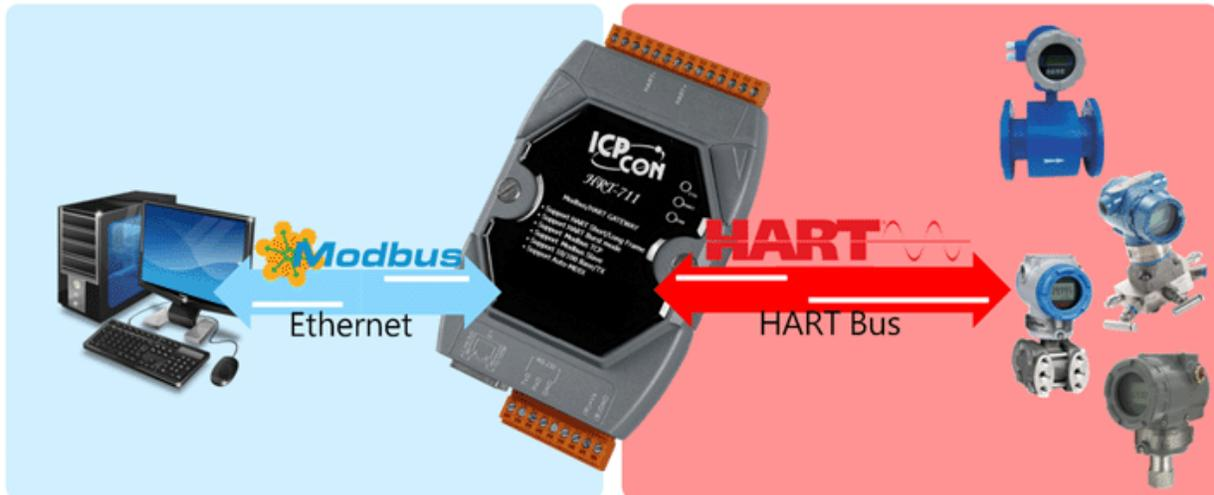
HART buses can operate in one of the two network configurations: point to point and multi-drop. In point to point mode, the analog signal is used to communicate one process variable and the digital signal gives access to secondary variables and other data that can be used for operations, commissioning, maintenance and diagnostic purposes. Only one HART slave device can exist in HART bus and the polling address must be zero.
