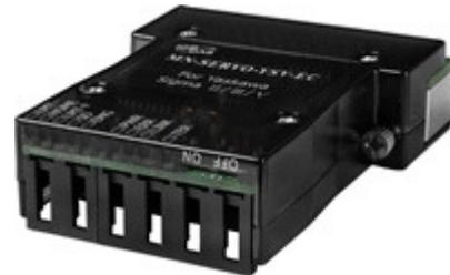
Slaves devices is based on RS-485 technology (Multi-drop, Half-duplex). This technology provides the advantage of simplifying connectivity of devices between remote distances while still offering high speed. Data transfer for the I/O modules is cyclical and time deterministic, so this mean that Motionnet devices can be used for other numerous industrial automation applications.
