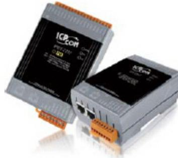
The ET-7200/PET-7200 module offers the most comprehensive configuration focused on meeting specific application requirements. It features a Built-in web server which allows configuration, I/O monitoring and I/O control by simply using a regular web browser. Remote control is as easy as surfing the Internet.
