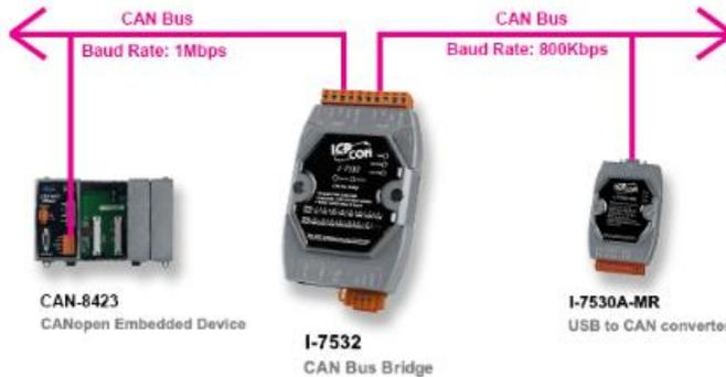
For these applications, we provide a CAN Bridge. The I-7532 can read a CAN message and rebroadcast it at a different baud rate. It can be used to isolate devices as well as extend the CAN Bus. The I-7532 supports both CAN 2.0A and CAN 2.0B so, it also works for J1939, DeviceNet and CANOpen networks.
