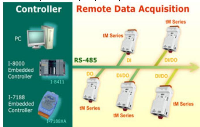
Our TM-AD5C module provides 5 Analog Input channels that can read in 4-20mA signals. Used in conjunction with a PC or PAC running datalogging or monitoring software, this can be a simple and cost effective way to monitor these signals.
